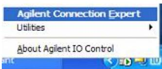
1. Open the Connection Expert utility by right clicking on the 'IO' icon in the system tray and selecting Agilent Connection Expert.
